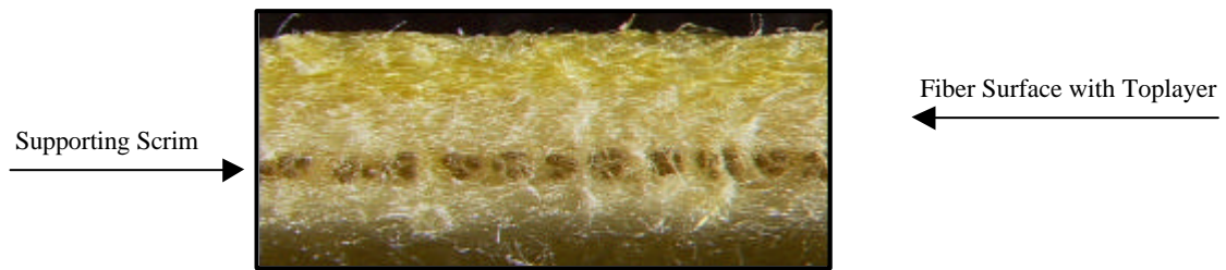
Figure 1: Cross-section of a textile filter medium
