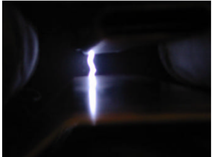
Fig. 13. Sparking at the Top of the Electrode System
