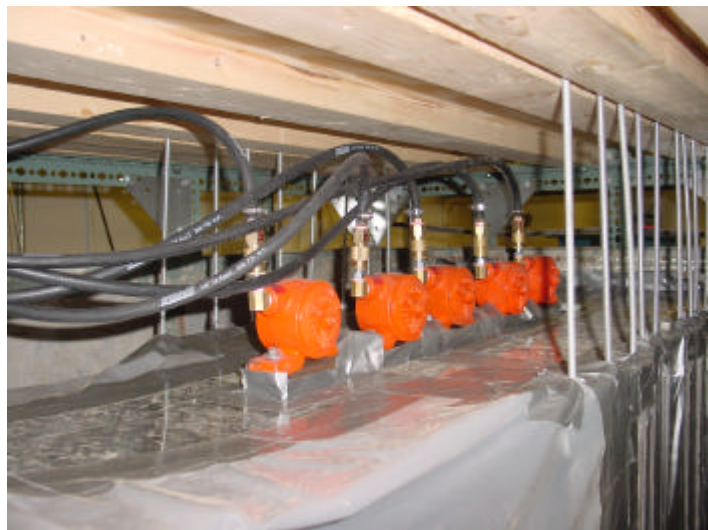
Fig. 8 Sets of screens suspended by bars on SEP sealing with pneumatic turbine shakers on top
