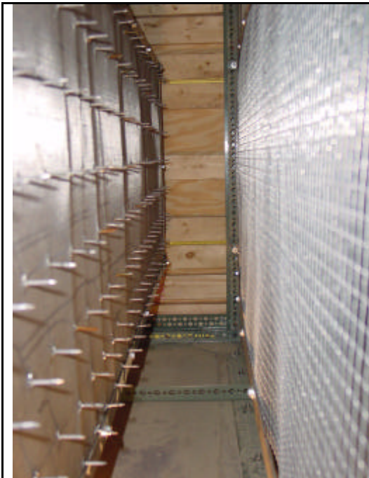
Fig. 7 Bottom view of the first grounded screen (right) and charging (left) screen
