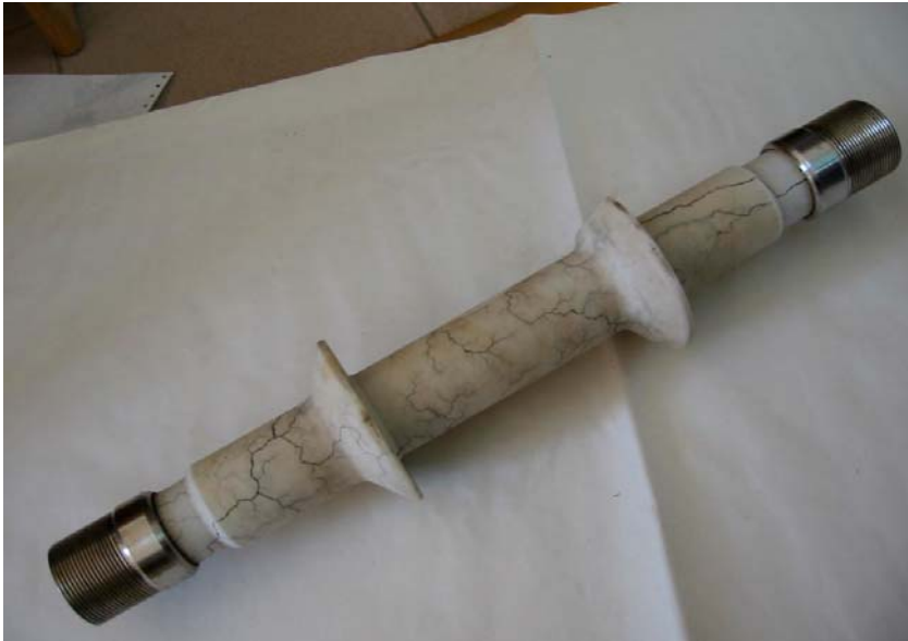
Fig. 2 Arborization trace on insulator surface
