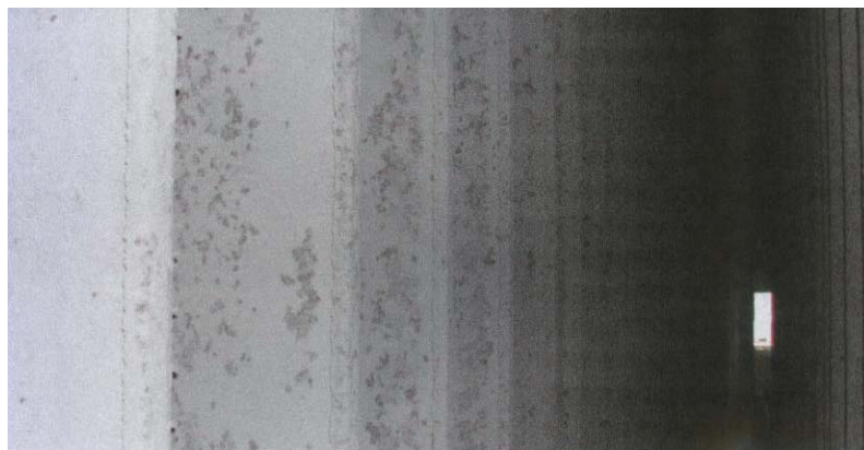
Fig. 7 Cleaned collecting plates after sonic rapping
